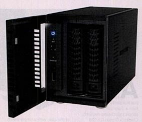
Another interesting feature is that the drive trays don't require tiny screws to hold the storage in place. Instead they've got a flexible plastic sleeve that extends out to capture the drive and then hold it firmly in place. These seem flimsy, but I prefer them
